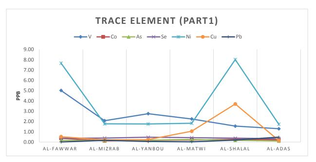
Figure 4.16 : Trace Elements (V, Co, As, Se, Ni, Cu and Pb) Concentrations in Springs water of Sarida Catchment
